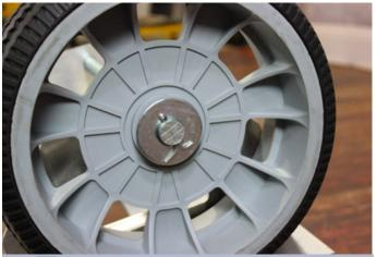
Insert a cotter pin, and using a needle nosed pliers, bend both sides outward to secure in place.
