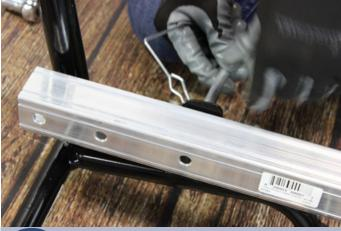
Pin the convertible handle into place to help stabilize the cart until the bolts are secured.
