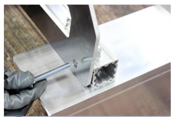
Lay your cart face down. Place a D bracket on the outside of the cart frame. Insert a bolt through the square hole on bracket and frame. Repeat for the 2nd square hole.
