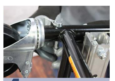
Stand the cart upright and insert the casters into the convertible handle. Use a snap pin to secure them in place.
