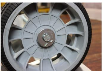
Insert a cotter pin, and using a needle nosed pliers, bend both sides outward to secure in place.
