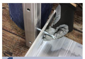
Center the foot plate onto the cart frame and align the holes on both. Insert bolts from front to back into each of the holes.
