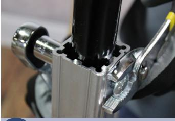
Finger tighten a lock nut onto the bolts.
