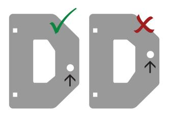
Make sure the D brackets are installed with the hole for the axle towards the bottom.
