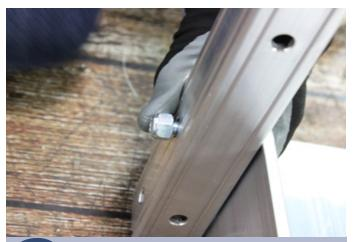
Thread a lock nut onto each bolt and finger tighten.
