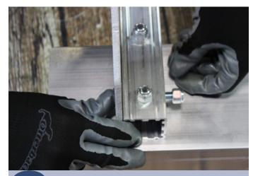
Install a lock nut on the bolt.
