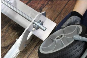
Slide 2 washers onto the axle, followed by one of the tires. Make sure the offset side of the tire is going towards the cart body.
