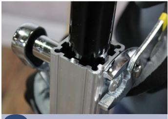
Finger tighten a lock nut onto the bolts. Then, using a socket 9/16" wrench and pliers, tighten the nuts down.
