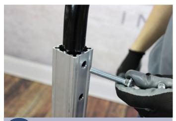
Insert a bolt through the cart frame and handle going from the outside of the frame to the inside.
