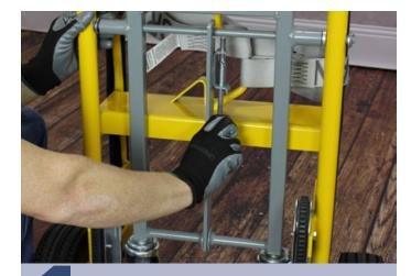
Pull the spring loaded lock down located on the back of the cart that holds the support bar in place.
