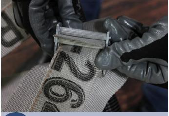
Lower the center roller and insert the strap back through, this time going above the roller.
