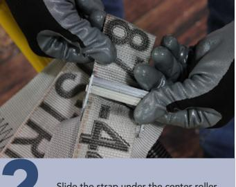
Slide the strap under the center roller.
